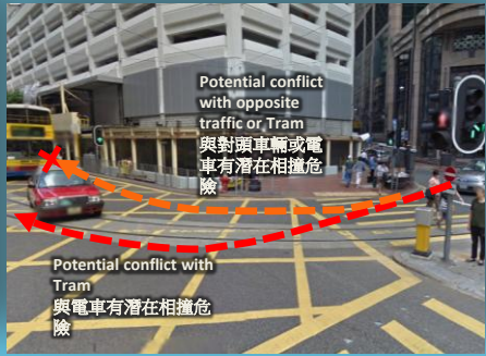
Large Vehicles Right Turn from Percival Street to Shape Street East Maneuvering Problems Cause Safety Issues. Potential Conflict of Vehicular Traffic and Tram 大型車輛較難從波斯富街右轉入駱克道導致安全問題。車輛與電車有潛在相撞危險
